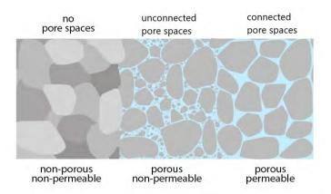
Figure 6-2 Porous vs Permeable Illustration
