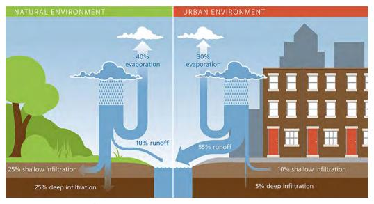
Figure 1-1 Impacts of urbanization on the hydrologic cycle
