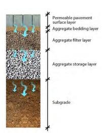
Figure 10-18 Typical pipeless drainage profile
