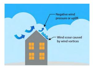
Figure 12-9 Effects of wind on roofs
