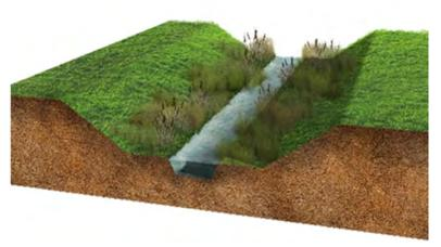
Figure 5-1 Two-stage channel
