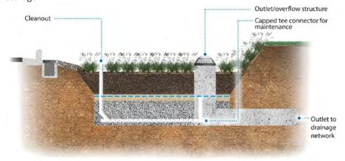
Figure 8-28 Bioretention cell with a saturated zone drainage profile Sealed Drainage Profile
