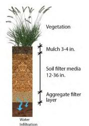
Figure 8-14 Typical Pipeless profile
