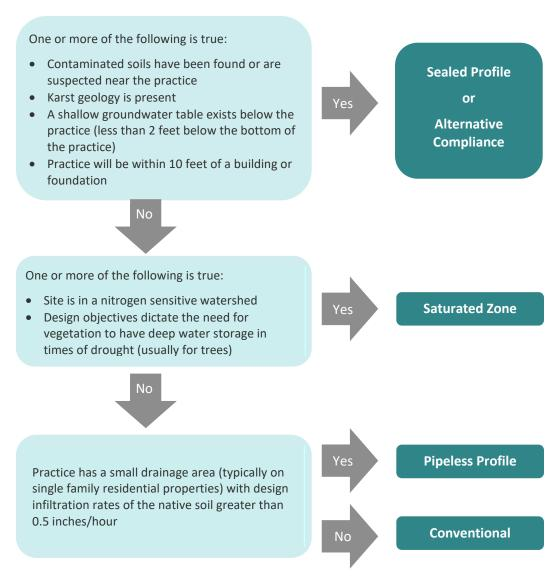
Figure 8-16 Drainage profile selection
