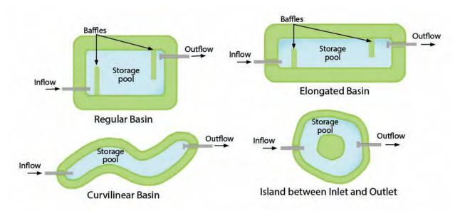
Figure 7-5 Methods of Increasing the Length-to-Width Ratio
