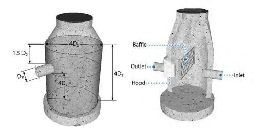
Figure 5-8 Inlet Structure with Sediment Sump
