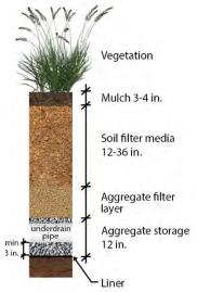
Figure 8-15 Typical sealed profile
