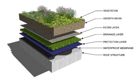
Figure 12-3. Single media assembly of a living roof
