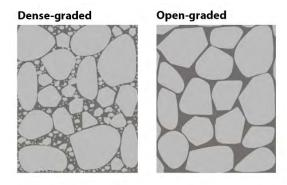
Figure 6-4 Packing of Aggregates Illustration
