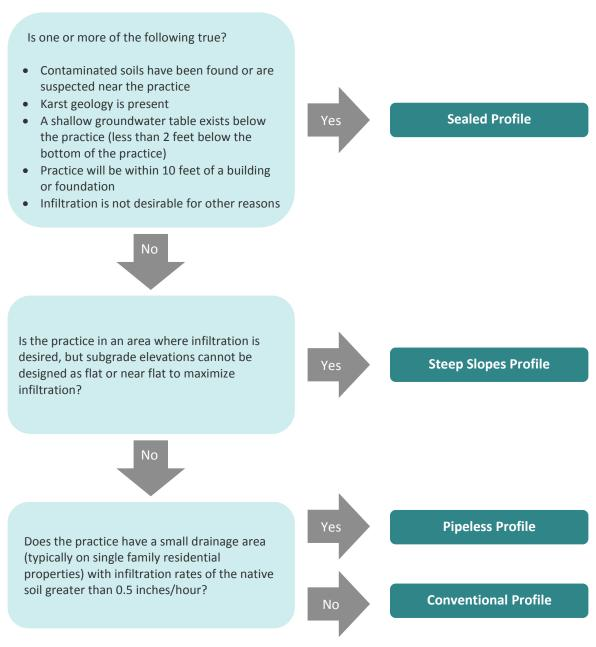
Figure 10-22 Drainage profile selection
