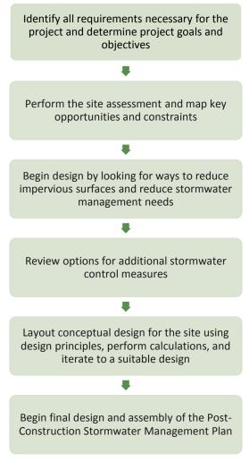
Figure 3-1 Integrated Site Design Process
