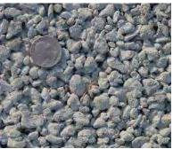
Figure 10-4 Example of Pervious Concrete
