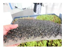
Figure 12-10 Living roof drainage layer
