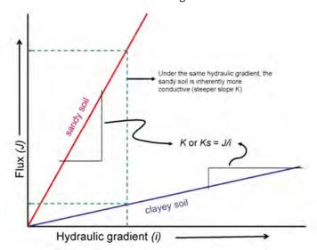
Figure 6-3 Relationship between specific discharge and hydraulic gradient
