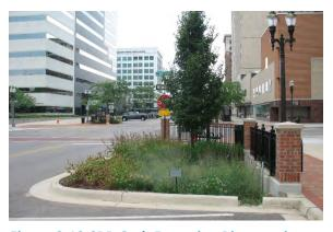
Figure 8-10 CBD Curb Extension Bioretention
