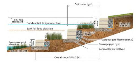
Figure 7-8 Terraced Side Slopes
