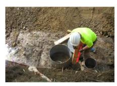
Figure 1-2 Soil infiltration test
