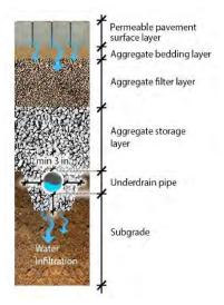
Figure 10-17 Typical conventional drainage profile
