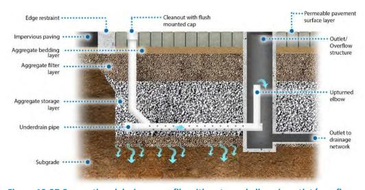
Figure 10-27 Conventional drainage profile with upturned elbow in outlet/overflow structure
