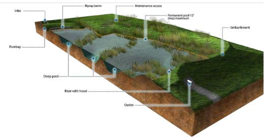
Figure 13-2 Example Stormwater Wetland Configuration
