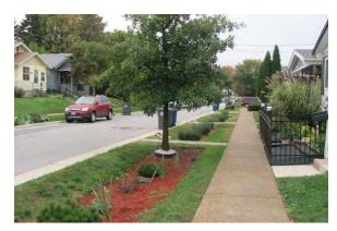
Figure 8-9 Linear Bioretention Along Roadway
