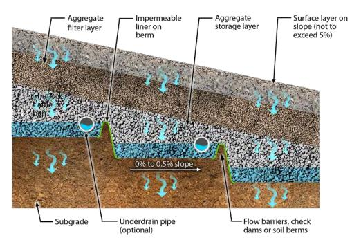
Figure 10-20 Steep slope drainage profile with subgrade terraces
