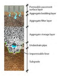
Figure 10-28 Sealed Drainage Profile
