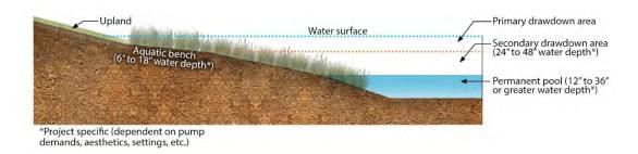
Figure 7-12 Hydraulic Profile of Detention Practice for Reuse
