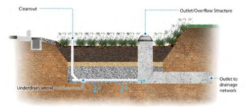
Figure 8-27 Bioretention cell with a conventional drainage profile
