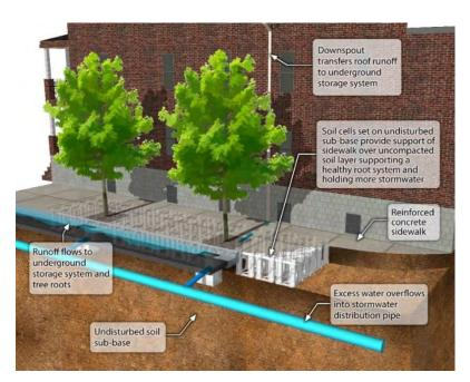
Figure 15-4 Typical suspended pavement system
