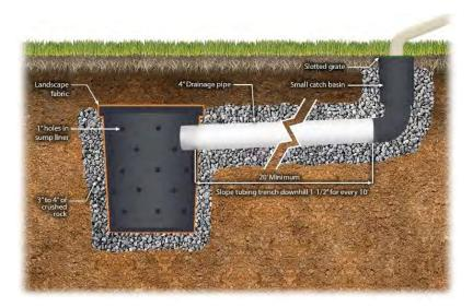
Figure 9-7 Dry well attached to roof downspout
