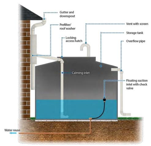
Figure 11-3 Dry conveyance inlet configuration
