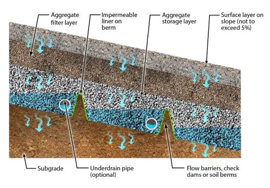
Figure 10-21 Steep slope drainage profile with sloping subgrade
