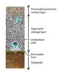
Figure 10-24 Single depth aggregate storage layer
