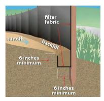
Figure 3-14 Silt fence
