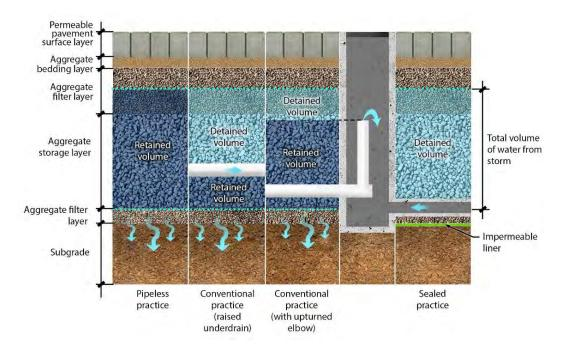
Figure 10-29 Cross-sections of drainage profiles
