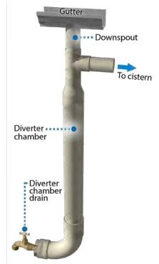
Figure 11-6 First-Flush Diverter
