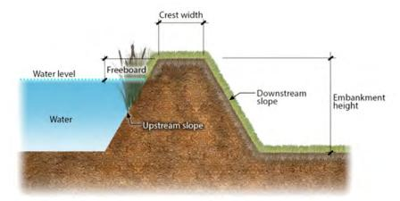
Figure 7-7 Embankment Illustration
