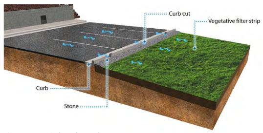
Figure 5-13 Typical Level Spreader
