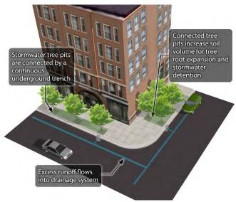
Figure 15-6 Interconnected tree pits
