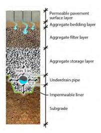
Figure 10-19 Typical sealed drainage profile
