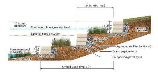
Figure 9-14 Terraced side slopes on an infiltration basin
