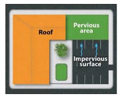
Figure 3-5 Disconnected impervious surface draining to lawn
