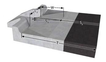
Figure 5-6 Depressed Curb Opening Cross Section
