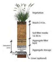
Figure 8-13 Typical Saturated Zone profile
