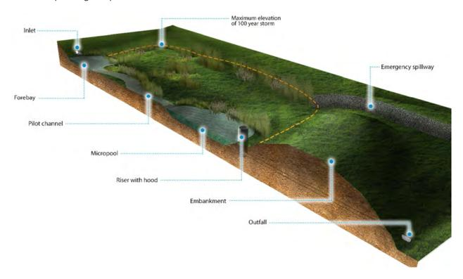
Figure 7-2 Extended Dry Detention with Micropool
