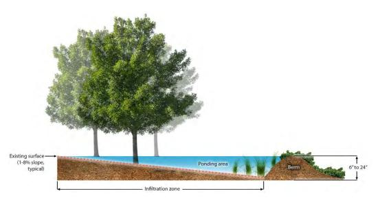
Figure 9-11 Section of an infiltration berm
