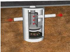
Figure 5-9 Gross Solids Removal Devices
