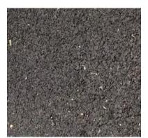
Figure 10-3 Example of Porous Asphalt
