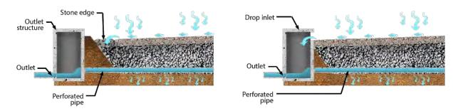
Figure 10-30 Permeable pavement overflow configurations
