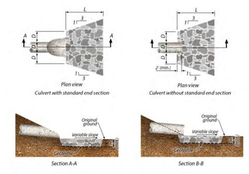
PROTECTIVE APRON AT CULVERT OUTLET WITHOUT DITCH
