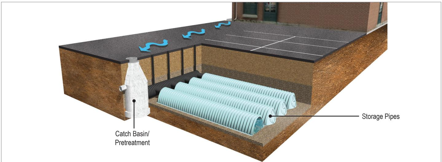
*Illustration of an underground pipe and chamber storage system under a parking lot*
