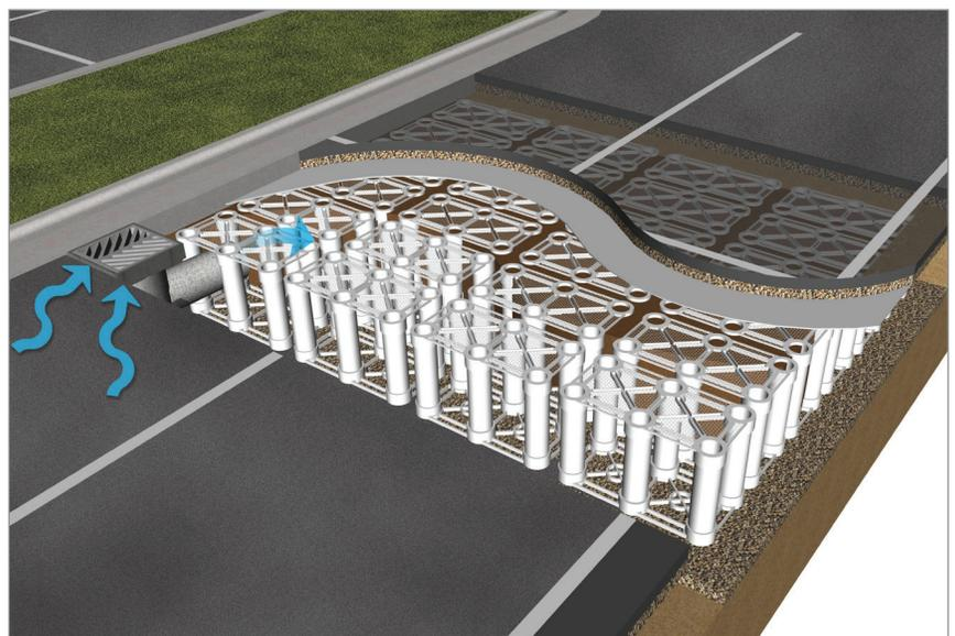
*Illustration of an underground plastic grid storage system under a parking lot*
